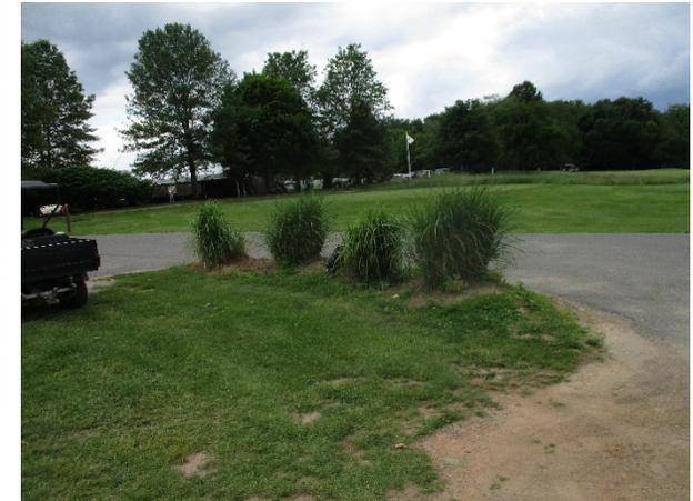
Near the entrance of the main building, a rain garden can be installed to collect water from the rooftop. Areas of the parking lot can be retrofitted with porous pavement to capture stormwater runoff from the parking lot. A preliminary soil assessment suggests that the soils have suitable drainage characteristics for green infrastructure.
